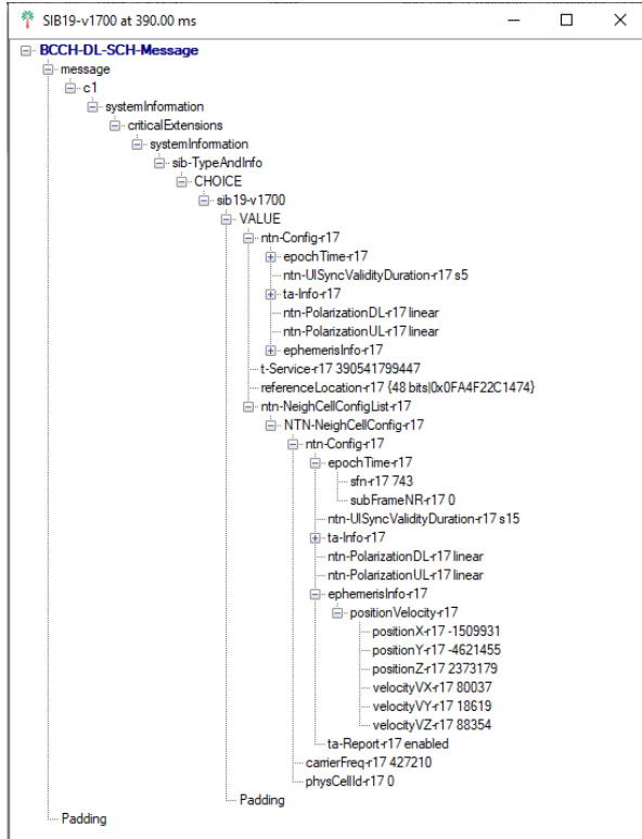
Figure 4. Data results using Keysight WaveJUDGE analyzer RF protocol sniffer for SIB19 satellite assistance information that includes a neighboring satellite
