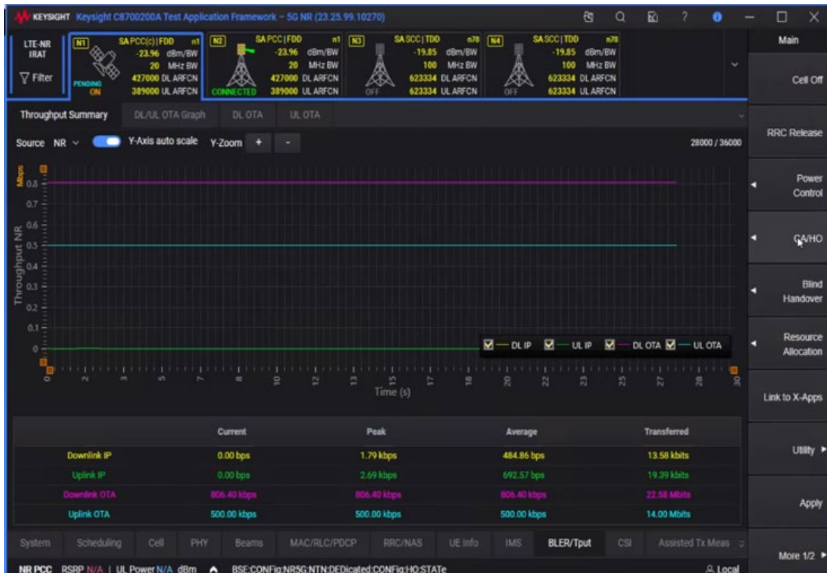
Figure 8. Keysight Test Application enabling mobility testing between TN and NTN
